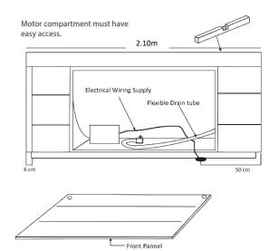
**IMPORTANT:** Important: The equipment must be connected to an exclusive and permanent power line capable to support installed power. Lighting and electrical receptacles must be located at least 1.5 meters from the equipment.
